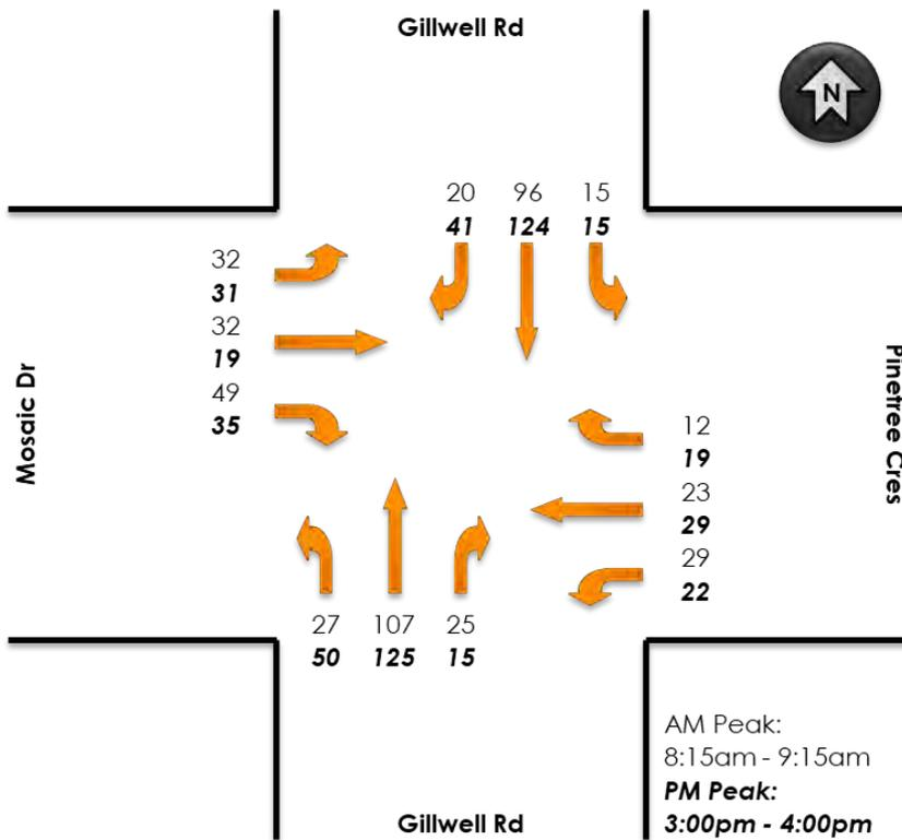
To assess the operation of the intersection the traffic volumes have been input into SIDRA Intersection, a traffic modelling software package.
