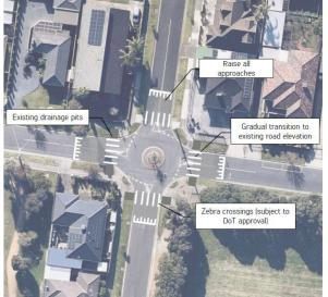
Figure 16. Boronia Street / Waratah Street raised roundabout (SALT 3, 2022)
