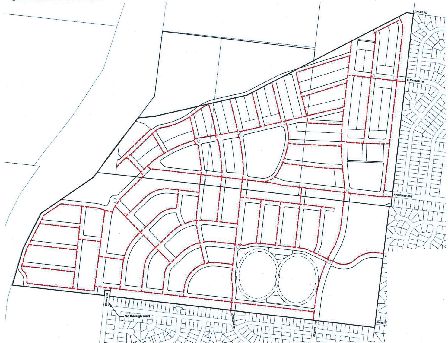
Figure 35: Telecommunications Conduit Plan
