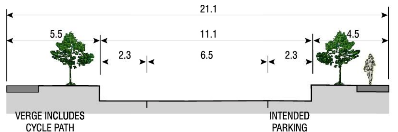
COLLECTOR TYPE A - ABUTTING ACCESS
