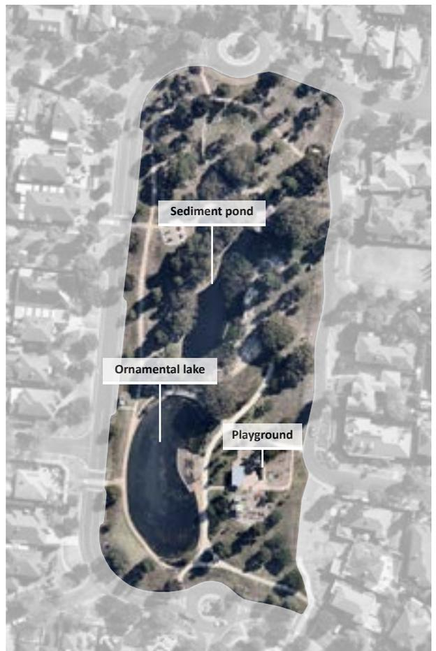
**Figure 3** At the Botanica Park in Bundoora, a WSUD asset (sediment pond) is complemented with pedestrian paths, a playground and a sheltered seating area that increase the park’s accessibility and frequency of use.
