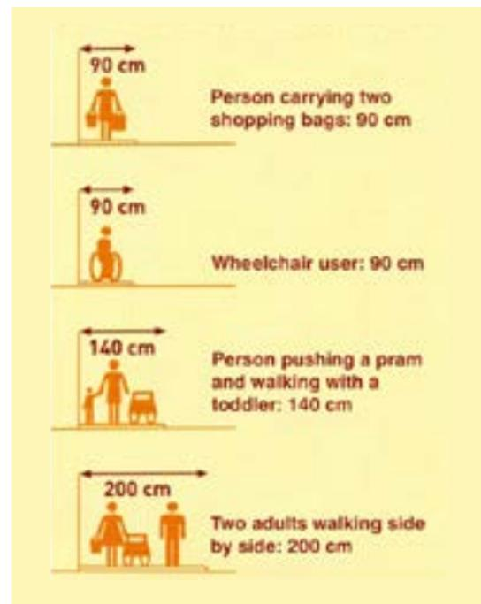
**Figure 13** Corridors for different widths of movement (Co-ordination Office for Planning and Construction Geared to the Requirements of Daily Life and the Specific Needs of Women).
