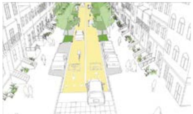
**Figure 4** Narrow lanes reduce speeds and minimise crashes by reducing the right-of-way and making drivers wary of traffic and adjacent users. Image taken from *Global Street Design Guide* (GDCI).
