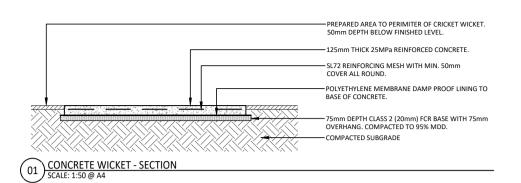
PRODUCT: NOT APPLICABLE SUPPLIER: NOT APPLICABLE MATERIAL AND STANDARD GREY CONCRETE WITH BASALT AGGREGATE, SMOOTH FINISH: TROWEL OR HELICOPTER FINISH. SYNTHETIC TURF TO BE 19mm SHORT PILE. FIXING / FOOTING: SYNTHETIC TURF TO BE FIXED TO MANUFACTURER'S SPECIFICATION ADDITIONAL OPTIONS: NOT APPLICABLE AUSTRALIAN STANDARDS: STANDARD DRAWING CROSS REFERENCES:
