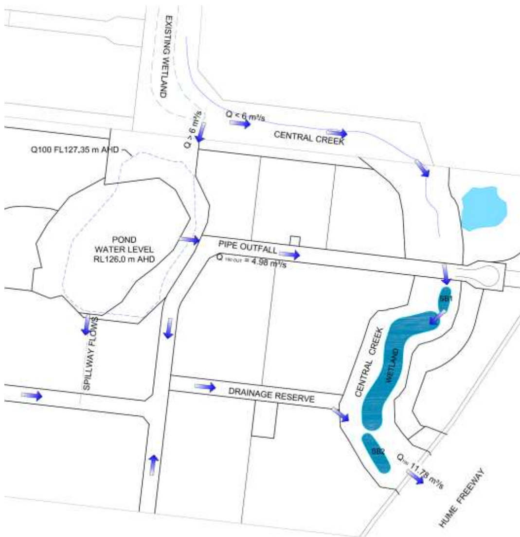
Figure 4.1 481 Cooper Street Epping Retarding Basin
