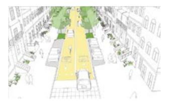
Figure 4 Narrow lanes reduce speeds and minimise crashes by reducing the right-of-way and making drivers wary of traffic and adjacent users. Image taken from *Global Street Design Guide* (GDCI). [h] Consider kerbless street design.
