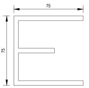
THIS SYMBOL SHALL BE MARKED ON THE FACE OF THE KERB IMMEDIATELY ABOVE THE POSITION WHERE AN ELECTRICAL SERVICE CONDUIT IS PLACED.
