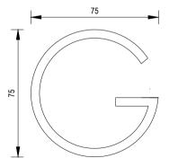
THIS SYMBOL SHALL BE MARKED ON THE FACE OF THE KERB IMMEDIATELY ABOVE THE POSITION WHERE A GAS SERVICE CONDUIT IS PLACED.
