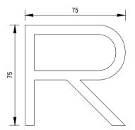
THIS SYMBOL SHALL BE MARKED ON THE FACE OF THE KERB IMMEDIATELY ABOVE THE POSITION WHERE A RECYCLED WATER SERVICE CONDUIT IS PLACED.
