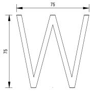
THIS SYMBOL SHALL BE MARKED ON THE FACE OF THE KERB IMMEDIATELY ABOVE THE POSITION WHERE A WATER SERVICE CONDUIT IS PLACED ACROSS THE ROADWAY.
