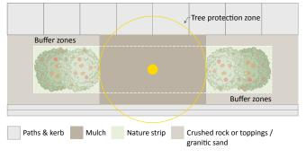
Figure 9 Example of nature strips that include crushed rock / granitic sand and mulch
